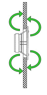
Stop of acoustic short-circuit with closed cabinet
