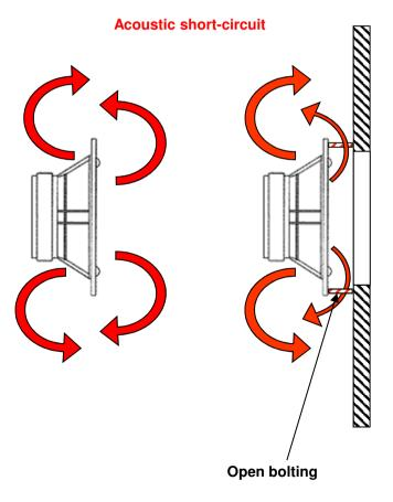
Stop of acoustic short-circuit with baffle
